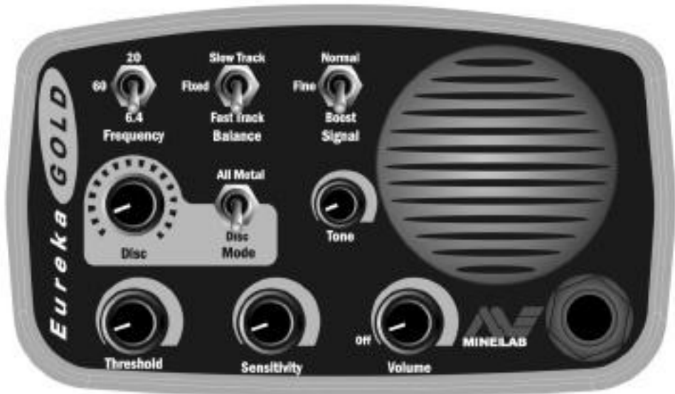
Figure 12 - The Eureka Gold Control Panel
